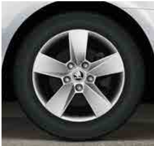
Alloy wheel 6.5J x 16" Ilias for tyre 205/55 R16 in silver design (5E0 071 496D 8Z8)
